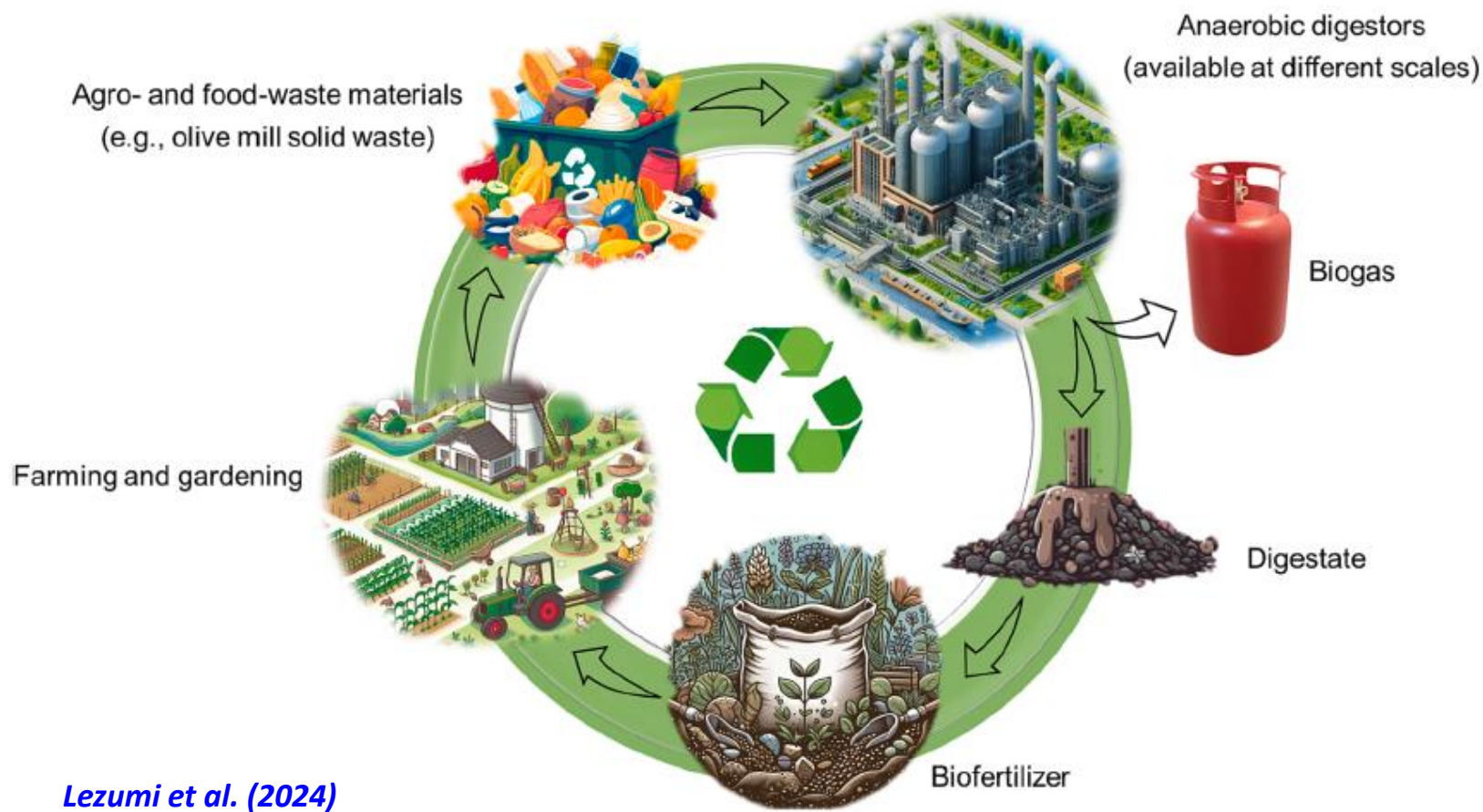
Fig. 2. Schematic process diagram of anaerobic digestion. It contributes to the implementation of circular economy concepts.
